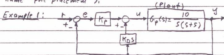
Obtain the values of gains  $K_p$  and  $K_D$  such that the closed-loop system has a characteristic equation of the form
